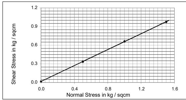
Cohesion  $C_u$  kg /cm<sup>2</sup>: 0.017 Angle Of Internal Friction  $\phi$ °: 32.64
