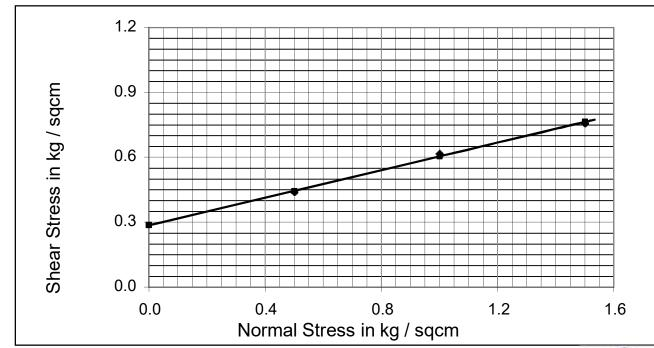
Cohesion  $C_u$  kg /cm<sup>2</sup>: 0.286 Angle Of Internal Friction  $\phi$ °: 17.65
