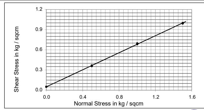
Cohesion  $C_u$  kg /cm<sup>2</sup>: 0.049 Angle Of Internal Friction  $\phi^{\circ}$ : 32.36
