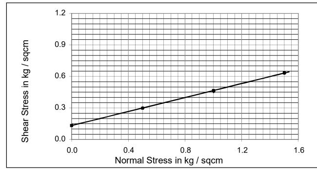
Cohesion  $C_u$  kg /cm<sup>2</sup>: 0.132 Angle Of Internal Friction  $\phi^o$ : 18.42
