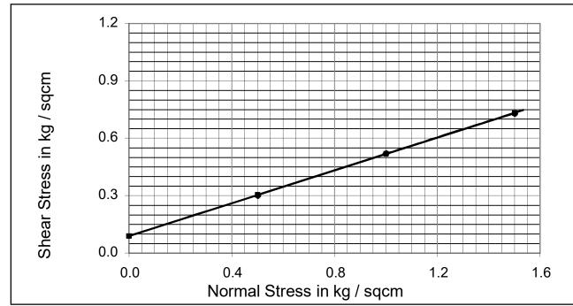
Cohesion  $C_u$  kg /cm<sup>2</sup>: 0.090 Angle Of Internal Friction  $\phi$ °: 23.18
