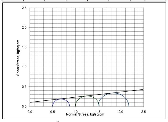
Cohesion:  $0.1 kg/cm^2$  Angle of internal friction,  $\phi$ : 7.52
