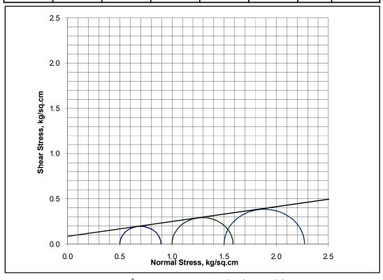
Cohesion:  $0.09 kg/cm^2$  Angle of internal friction,  $\sigma$ : 9.09
