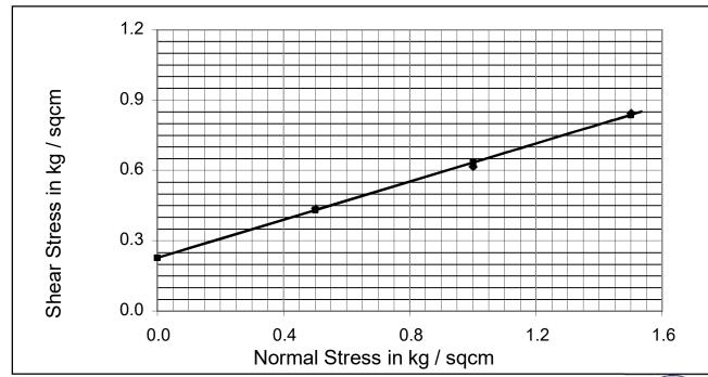
Cohesion  $C_u$  kg /cm<sup>2</sup>: 0.227 Angle Of Internal Friction  $\phi$ °: 22.10
