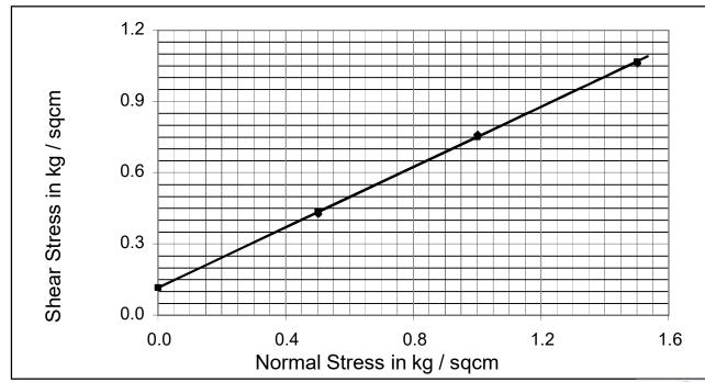
Cohesion C<sub>u</sub> kg /cm<sup>2</sup>: 0.116 Angle Of Internal Friction φ°: 32.39
