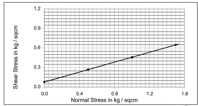
Cohesion  $C_u$  kg /cm<sup>2</sup>: 0.078 Angle Of Internal Friction  $\phi^o$ : 20.80
