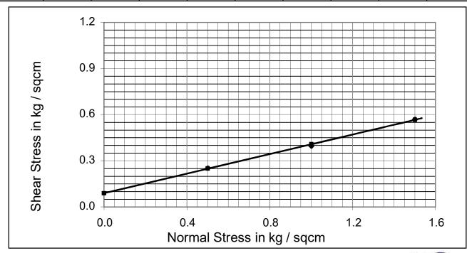
Cohesion  $C_u$  kg /cm<sup>2</sup>: 0.090 Angle Of Internal Friction  $\phi^{\circ}$ : 17.60
