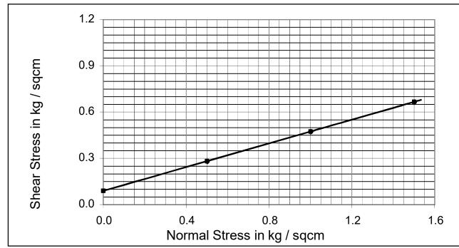
Cohesion  $C_u$  kg /cm<sup>2</sup>: 0.089 Angle Of Internal Friction  $\phi$ °: 21.05
