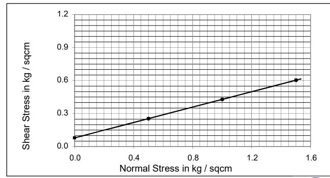
Cohesion  $C_u$  kg /cm<sup>2</sup>: 0.079 Angle Of Internal Friction  $\phi$ °: 19.23
