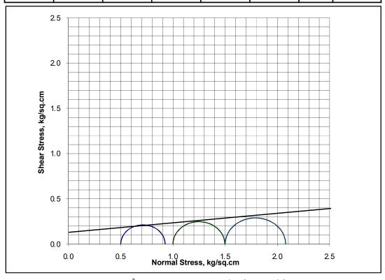
$kg/cm^2$ Angle of internal friction, ø: Cohesion: 0.13 5.71
