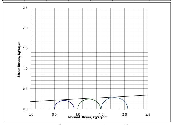
Cohesion:  $0.18 \text{ kg/cm}^2$  Angle of internal friction,  $\emptyset$ : 3.43
