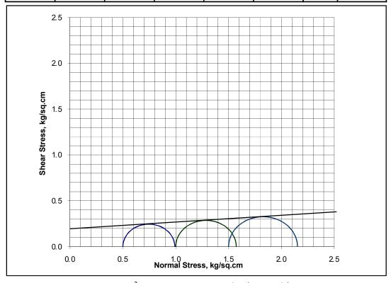
Cohesion:  $0.20 \text{ kg/cm}^2$  Angle of internal friction,  $\emptyset$ : 4.12
