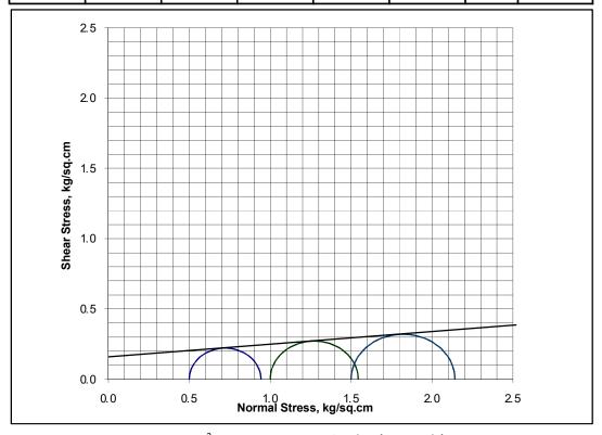
Cohesion:  $0.16 \text{ kg/cm}^2$  Angle of internal friction,  $\emptyset$ : 5.03
