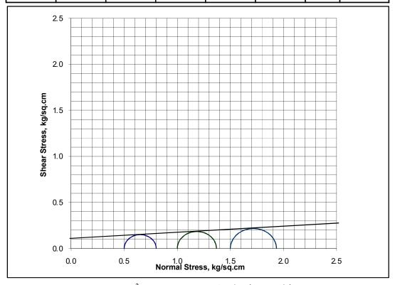
Cohesion:  $0.11 \text{ kg/cm}^2$  Angle of internal friction,  $\emptyset$ : 3.66
