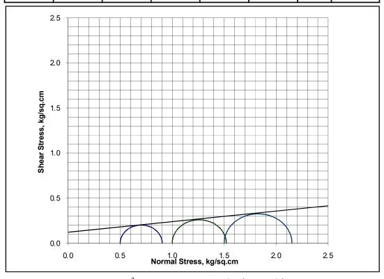
Cohesion:  $0.12 \text{ kg/cm}^2$  Angle of internal friction,  $\emptyset$ : 6.62
