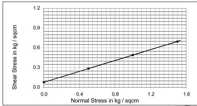
Cohesion  $C_u$  kg /cm<sup>2</sup>: 0.079 Angle Of Internal Friction  $\phi$ °: 22.41
