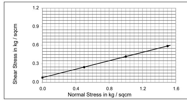
Cohesion  $C_u$  kg /cm<sup>2</sup>: 0.076 Angle Of Internal Friction  $\phi$ °: 18.84
