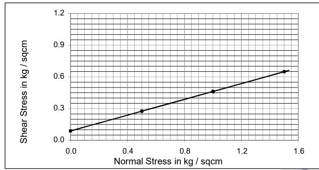
Cohesion  $C_u$  kg /cm<sup>2</sup>: 0.088 Angle Of Internal Friction  $\phi$ °: 20.5
