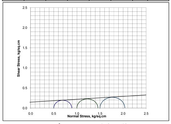
Cohesion:  $0.15 \text{ kg/cm}^2$  Angle of internal friction,  $\emptyset$ : 3.89
