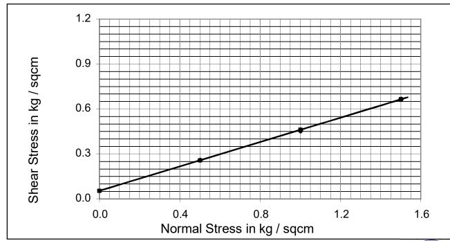
Cohesion  $C_u$  kg /cm<sup>2</sup>: 0.054 Angle Of Internal Friction  $\phi$ °: 22.10
