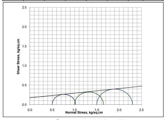
Cohesion:  $0.18 \text{ kg/cm}^2$  Angle of internal friction,  $\emptyset$ : 6.62
